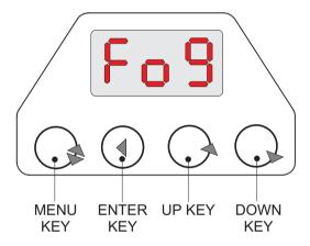
The message displayed will depend on the operating mode of the machine at the time. However, pressing the menu key at any time will cause the display to go into the edit mode, allowing the operating parameters to be adjusted. After approximately 15 seconds since the last keystroke, the display will leave the edit mode and revert to displaying the current status information.
